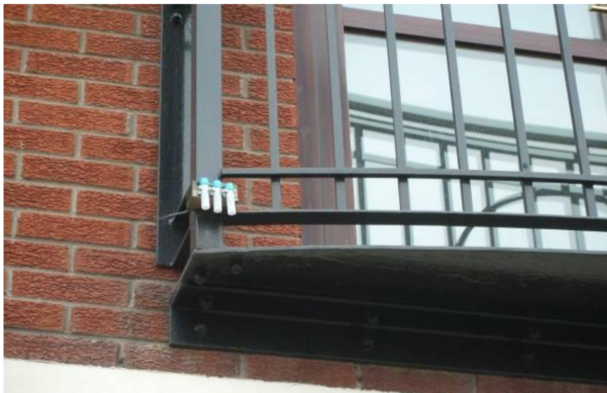
Figure 2.9 Picture of NO 2 Tubes on AQMA Normandy Court Dundonald
