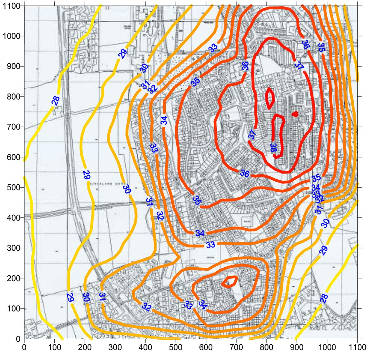
**Figure 7.3e – 99.9 percentile 15 minute mean SO<sub>2</sub> concentrations for Ballysally**
