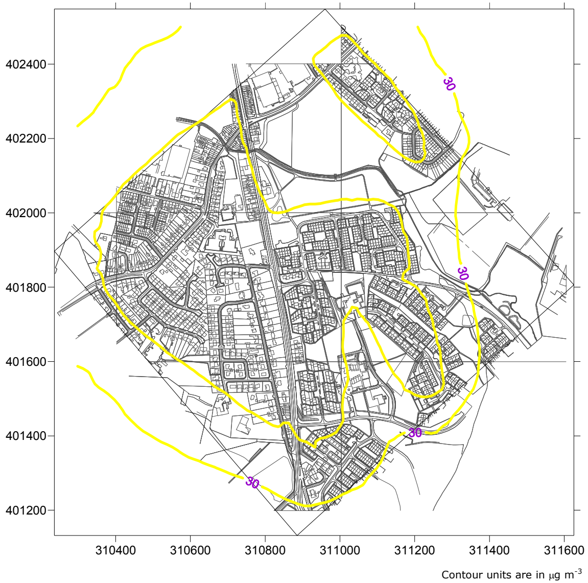
Figure 4.11 Ballee – 2004 PM 10 24h mean corrected modelled results (the bias factor was determined using monitoring data from Carrickfergus BC).
