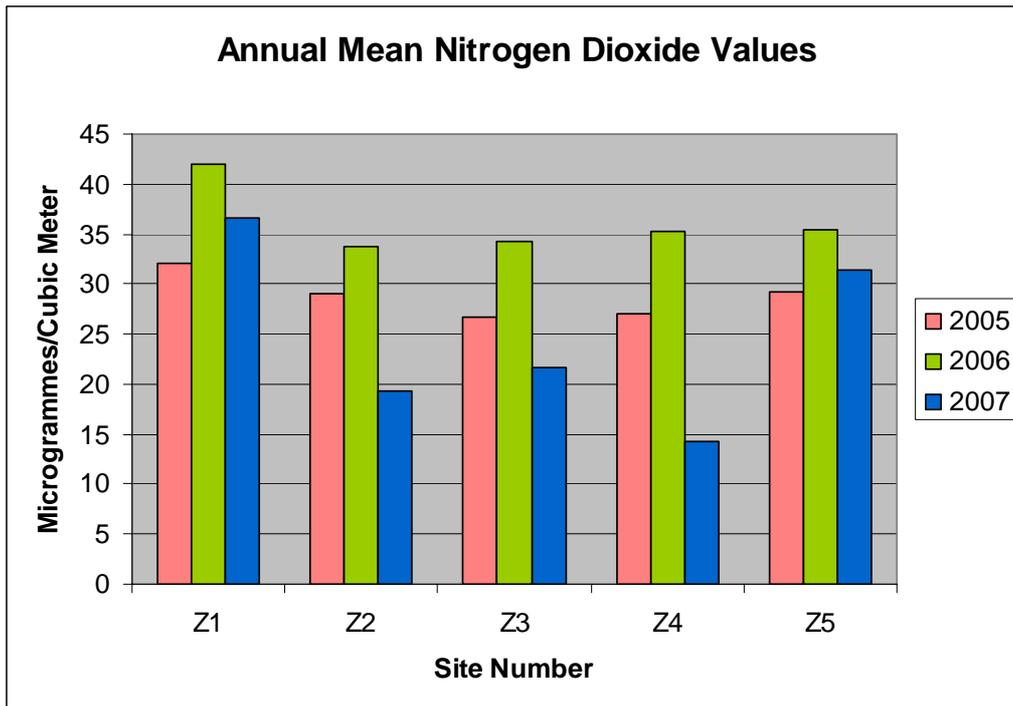
As Z1 has shown a consistently higher reading than the rest, the tube at this site has been moved to a more representative position for residential exposure. A further two tubes have also been placed in Moneymore along the main traffic thoroughfare to ensure that the levels obtained are representative of air quality in the area.
