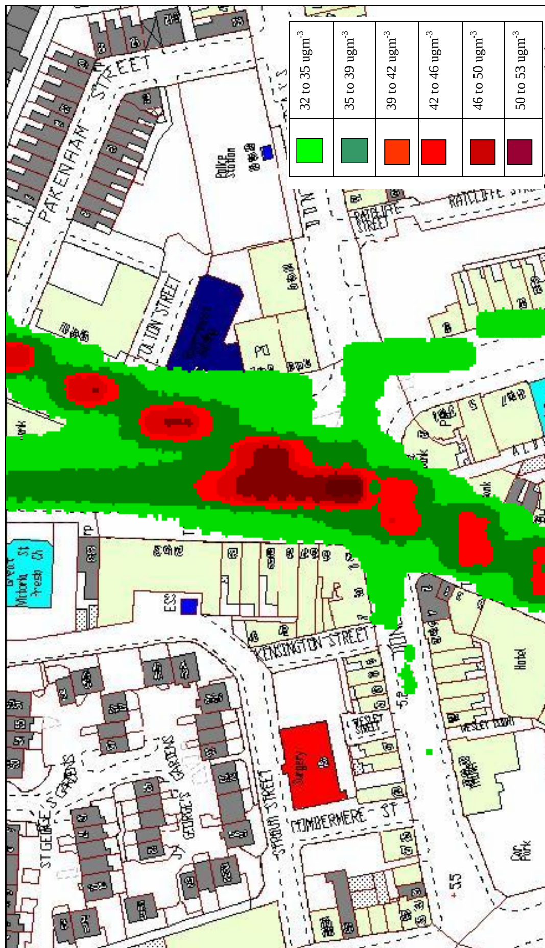
Figure 6. Junction 3, Modelled annual mean nitrogen dioxide concentrations, 2006.
