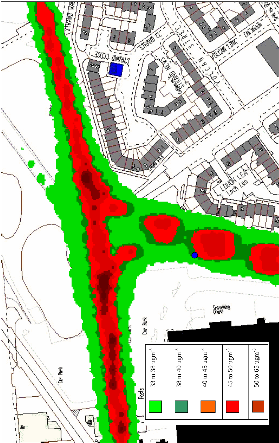
Figure 3. Junction 1, Modelled annual mean nitrogen dioxide concentrations, 2006.
