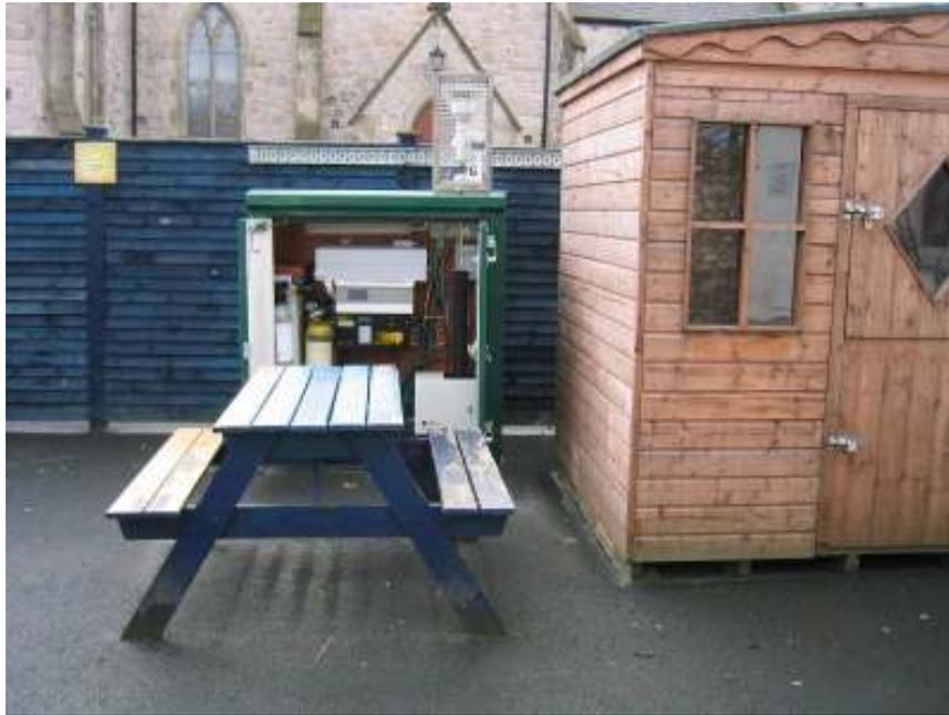
Photograph 3 – Showing Real time monitoring equipment for SO<sub>2</sub> and PM<sub>10</sub> located at Gortalowry House, Cookstown.
