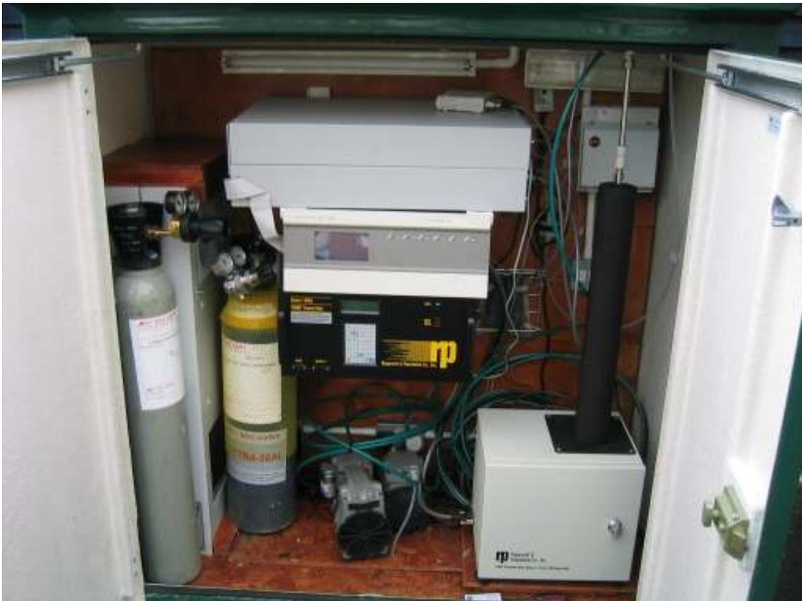
Photograph 2 – Showing TEOM Ambient Particulate (PM<sub>10</sub>) Monitor Located at Gortalowry House, Cookstown
