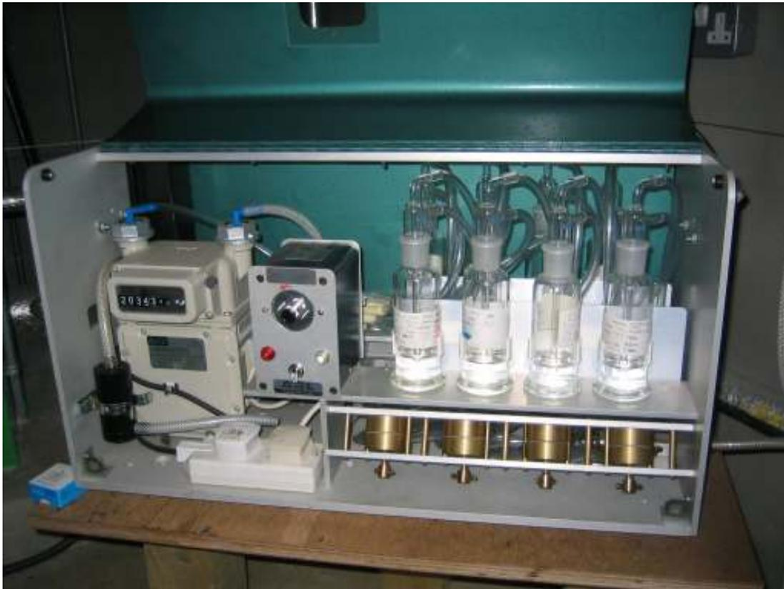
**Fig 7. Sulphur Dioxide Bubbler Site**
