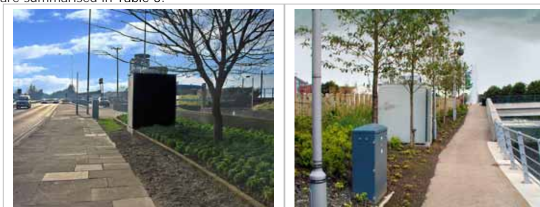
Figure 2 North Down Holywood (left) and Lisburn Civic Centre (right) automatic monitoring stations
