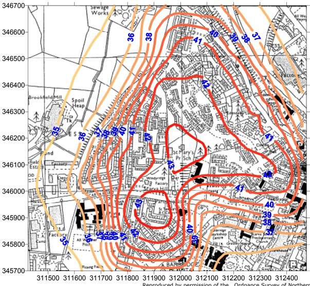
Figure 6.5. A contour plot of  $PM_{10}$  concentrations predicted by the ADMS model relevant to the 24 hour objective.
