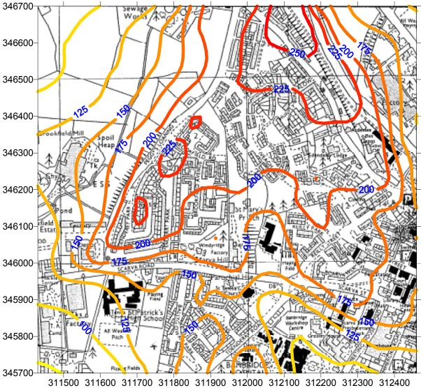
Figure 6.4. A contour plot of SO<sub>2</sub> concentrations predicted by the ADMS model relevant to the 15 minute mean.
