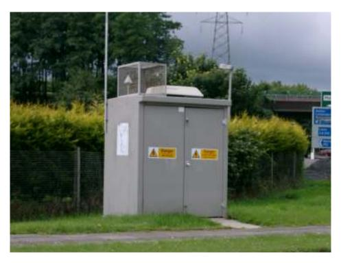
The pollutant measured at both the stations is oxides of nitrogen.
