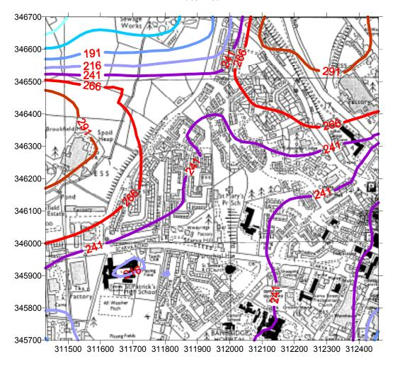
Figure 5.4. A contour plot of concentrations predicted by the ADMS model relevant to the 15 minute mean.
